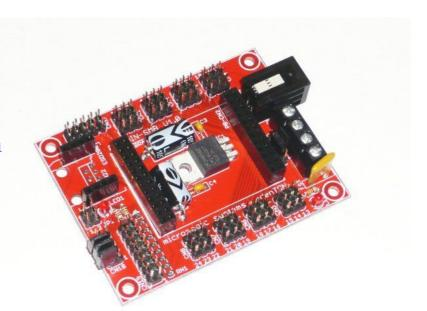
This motherboard is designed to take the p.Brain-ds24 robot controller, and will not function as a stand alone unit.
