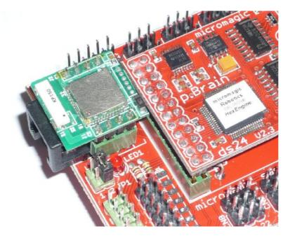
Image showing ESD200 fitted into  $4 \times 1~0.1''$  pitch header sockets. CN22b RJ11 6/6 has also been fitted below the ESD200 to facilitate ICSP facility. CN22b is not fitted as standard, and is not necessary for the ESD200 operation.
