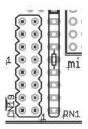
This socket is provided for the user to add a SIL resistor net for a different pull up resistance value if required. The dsPIC33 already has pull up capabilities on ANA0 through to ANA5.
